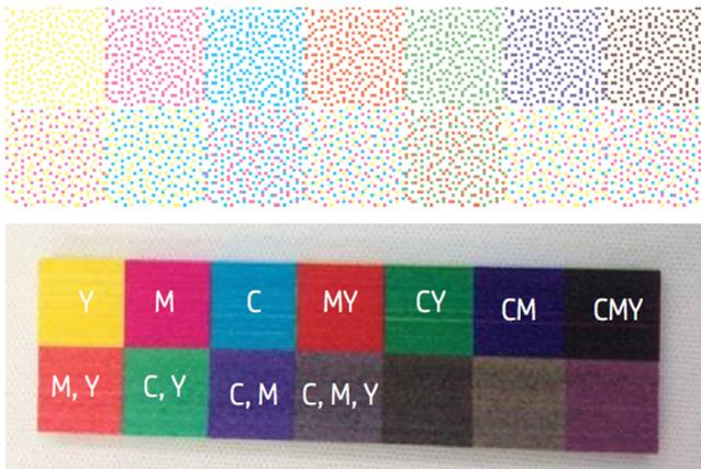
Fig. 6: Simple Mvocs, shown as the input halftone (low resolution single slice, top) and as the object printed on a prototype testbed (bottom).
