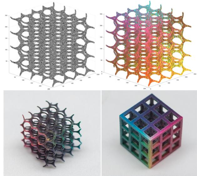
Fig. 5: Structural PARAWACS3D halftone matrices applied to a simple cube object with smooth color gradients. Top row: visualization of halftone matrix (left) and final halftone (right), bottom row: printed object photos.
