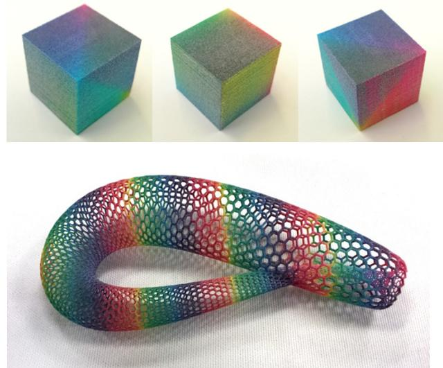
Fig. 7: An RGB cube (top) and a Klein bottle model, processed using the LUT shown in Tab. 2. The input for this object in geometric terms is a plain cube and the Klein bottle [23], while in the case of the cube, every location  $[x, y, z]$  has a unique RGB color specified, proportionally representing all possible RGB values. The Klein bottle instead used a color transitioning map, also throughout the object.
