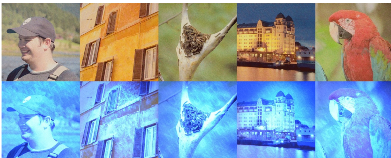
Figure 6. Watermarked test images using \alpha = 3 , as seen under D50 illumination (top row) and indoor office light plus UV flashlight from approximately 10 cm distance (bottom row).
