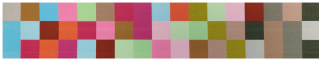
Figure 6. Printed halftone patterns ordered left to right from low to high by (top) perceived grain, (middle) grain predicted from NPacs and (bottom) grain predicted from YN-filtered halftones.
