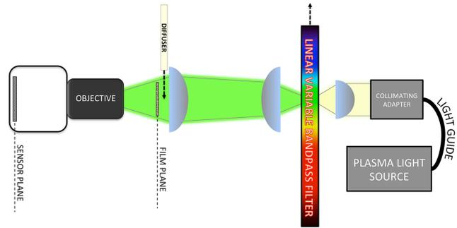
Figure 2. The measuring setup adopted for the acquisition of the multispectral images
