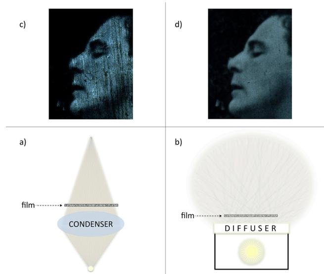
Figure 1. *Below*: Schemes of directed (a) and diffuse (b) illuminations. *Above*: Corresponding images of a photographic film (c and d respectively). The film is a print of “Das Cabinet des Dr. Caligari” (R. Wiene, 1920) that underwent metallic toning.
