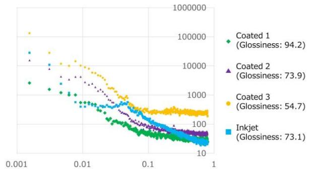
Figure 15. The power spectral density of measured surface topography.
