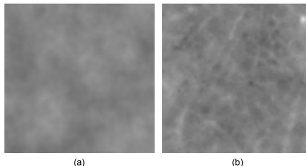
Figure 1. The two kinds of depth maps. (a) is the Perlin noise. (b) is measured surface topography.
