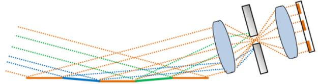
Figure 8. The ray trajectory on the telecentric optical system.
