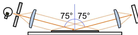
Figure 2. The apparatus diagram of the collimator optical system. The lighting and viewing angle are set to be 75 degree.
