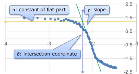
Figure 10. The wiener spectrum of the spatial frequency property of the unevenness and calculated feature values from the wiener spectrum.
