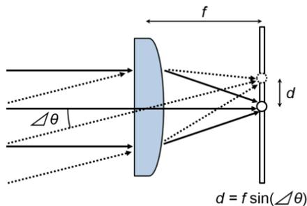
**Figure 3.** Schematic diagram of a collimator lens system. The focal point distance ( $d$ ) can be calculated from the focal length( $f$ ) and the difference of angle( $\Delta\theta$ )
