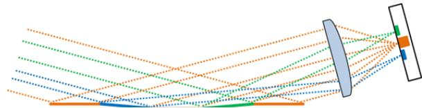
**Figure 4.** The ray trajectory on the collimator optical system.
