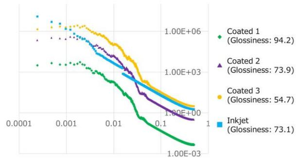
Figure 16. The power spectral density of estimated surface topography.
