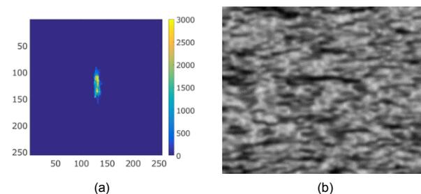
Figure 12. The example of simulation results measured Perlin noise surface topography on the computer simulation. (a) is measured with the collimator optical system. (b) is measured with the telecentric optical system.
