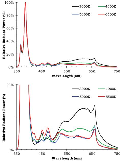
Figure 1 The relative spectral power distribution of the four lighting conditions.
