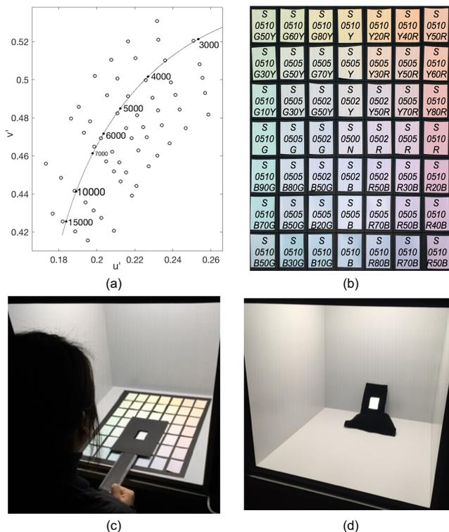
**Figure 2.** Experiment setting. (a) The illuminant used in the experiment plotted in CIE 1976  $u'v'$  space; (b) The NCS samples used in the experiment part 1; (c) The experiment situation of part 1; (d) The experiment situation of part 2;
