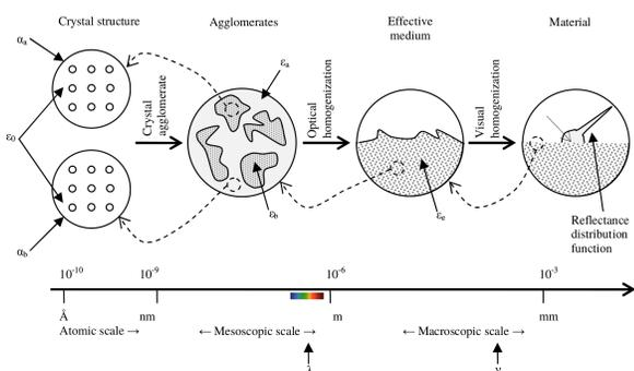
**Figure 2.** The links between the successive scales of representation are presented in a schematic view from nanoscopic (crystallographic properties) to macroscopic visual properties.
