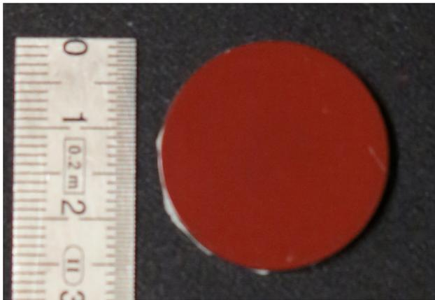
**Figure 7.** We prepared several samples of embedded hematite pigments in several crystallographic shapes at the nanoscale and several concentrations (5 - 7 and 10%). Here is a nano pseudocubes powder inside an epoxide resin for a 7% volumetric pigments concentration.
