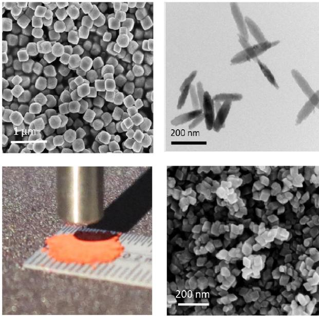
**Figure 9.** Top left: nano-pseudocubes. Top right: nano rods. Bottom left: spectrophotometric measurement of the nano pseudo-cubes powder produced for making a red-orange paint. Bottom right: rhombohedral crystals.
