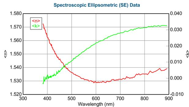
**Figure 6.** The binder optical characteristics. Measured by spectroscopic ellipsometry, the optical data  $n$  and  $k$  exhibit a greater transparency in the blue region of the spectrum.
