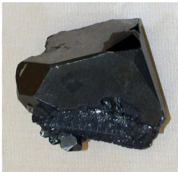
**Figure 3.** A macroscopic sample of hematite having a sub-metallic lustre, displayed in the Mineralogy collection at Ecole des Mines de Paris, used for easily determine the dielectric tensor components by spectroscopic ellipsometry.
