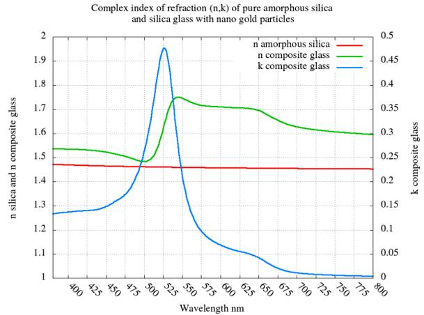
**Figure 1.** Complex index of refraction of a silica glass including nano particles of gold at a volumetric concentration of 0.05% compared to pure amorphous silica. Notice the very important variation in the optical index not only in the neighbourhood of the absorption wavelength band.
