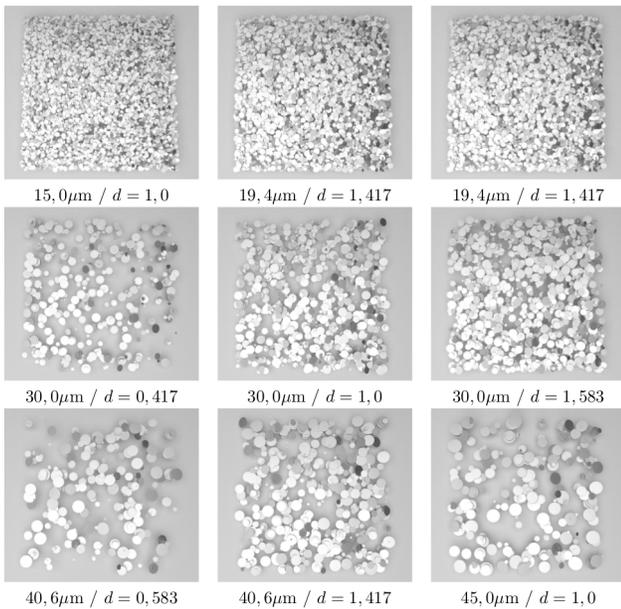
**Figure 10.** A set of generated density maps containing several metallic flakes with various diameters and radii. The simulated sample of painted plates were obtained in the size of 15cm x 10cm including 332 x 240 microstructures.
