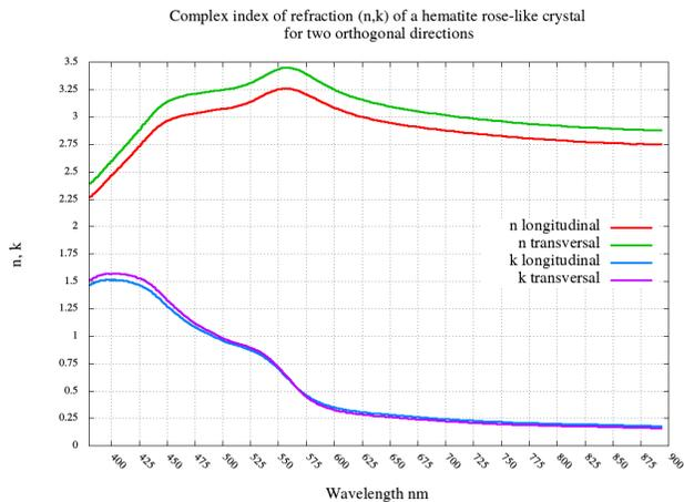
**Figure 5.** Comparison of the complex indices of refraction of a rose-like hematite crystal measured for two orthogonal directions. The difference in absorption (curves "k") is very weak while it is not so negligible for the optical index. We nevertheless use a mean optical index.
