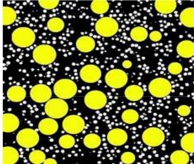
**Figure 8.** From a statistical analysis of a SEM image of a real paint made of nano pseudocubes are extracted several parameters useful for a mathematical modeling: exclusion zones (yellow disks), concentration, contacts and alignments, etc. Image size:  $20\mu\text{m} \times 20\mu\text{m}$ .
