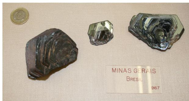
**Figure 4.** Anisotropic lamellar hematite crystals in rose-like shape having a high metallic lustre. Ellipsometric spectroscopic measurements were made in two independent directions taken in the petal plane, except in the third dimension (thickness) where no measurements were possible. The difference in optical properties is not very significant when used at nano or microscopical level. Museum of Mineralogy of Ecole des Mines de Paris.
