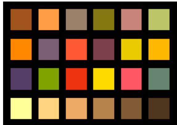
Figure 6. Colors of figure 3 (F12) transformed with a LUT optimized for ColorChecker colors from camera RGB under illuminant F12 to standard observer simulation based sRGB colors. Reference colors at top row of each patch same as in figure 3 (F12).
