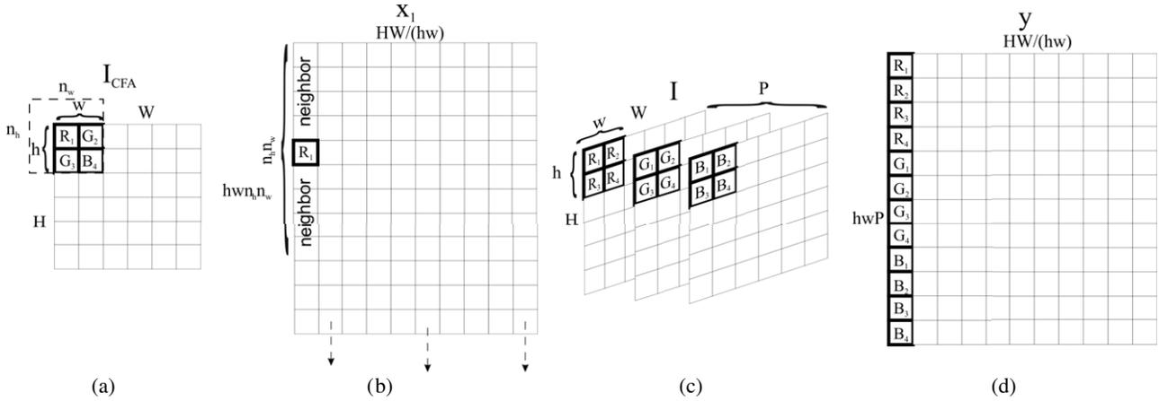
Figure 1. Detail of the unfolding of images into vectors (a) Mosaiced image  $I_{CFA}$  with a neighborhood shown (b) Unfolding of the mosaiced image into matrix  $x_1$  (c) Color image  $I$  (d) Unfolding of the color image into matrix  $y$ .
