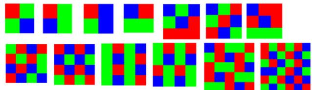
Figure 3. Different CFA pattern used for comparison. From left to right top row, Bayer,  $2 \times 2$  #1,  $2 \times 2$  #2,  $2 \times 2$  #3,  $3 \times 3$  #1,  $3 \times 3$  #2,  $3 \times 3$  #3, bottom row,  $4 \times 4$  #1,  $4 \times 4$  #2, Yamanaka,<sup>14</sup> Lukac,<sup>13</sup> Holladay half-tone,<sup>30</sup> CNRS.<sup>15</sup>
