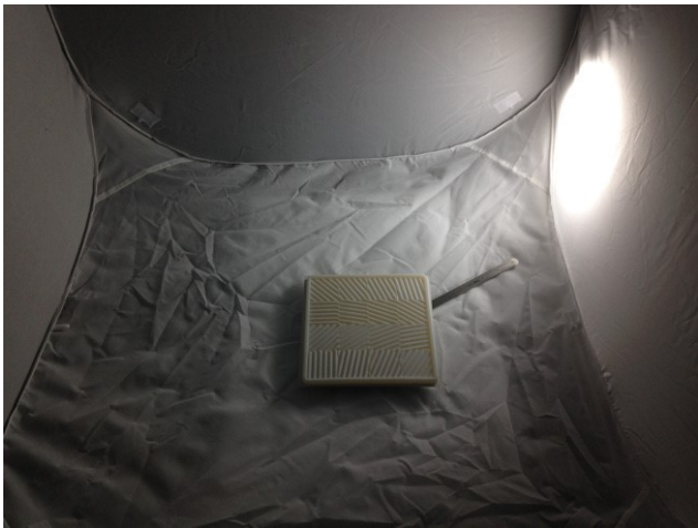
Figure 4. Experiment two used the same lighting and positioning shown in figure 2 but in this case the target is placed within a diffusing box and the illumination is outside of this box.
