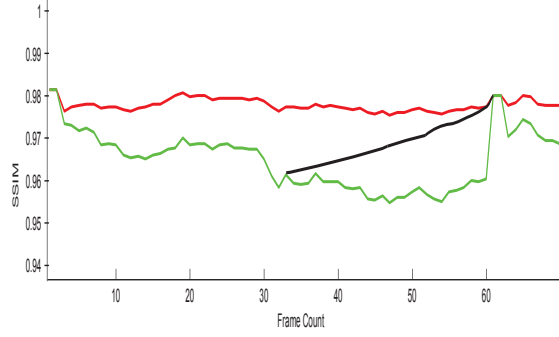
Figure 2. Idealized representation of how drift correction would work. The black line represents the drift correction's impact on the SSIM measure
