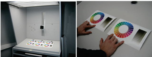
Figure 5. Setup of the rank-order experiment (left) and the pair-comparison experiment (right). Both are carried out under D50 norm-light. The instructions were given in written form.
