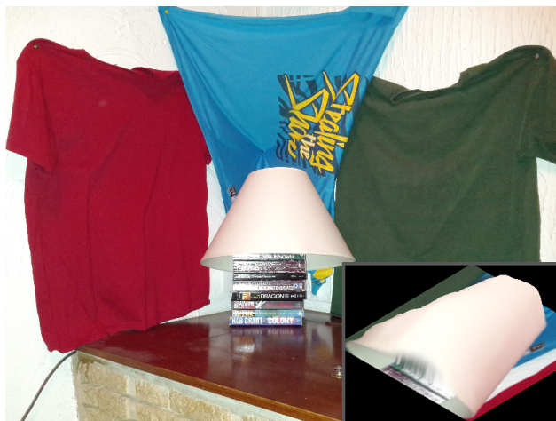
Figure 6. Preliminary results demonstrating the resilience of our method to less ideal environments. A lampshade illuminated by indirect illumination from three t-shirts. Shape was recovered from a single rendered image (i.e. jpg) rather than linear raw data with good accuracy.
