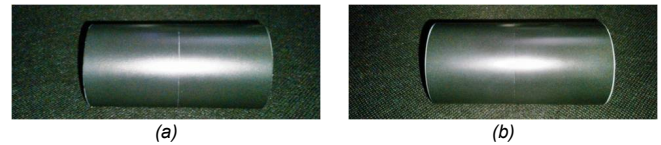
Figure 3. Two kinds of object. (a) is wrapped by high gloss paper. (b) is wrapped by low gloss paper
