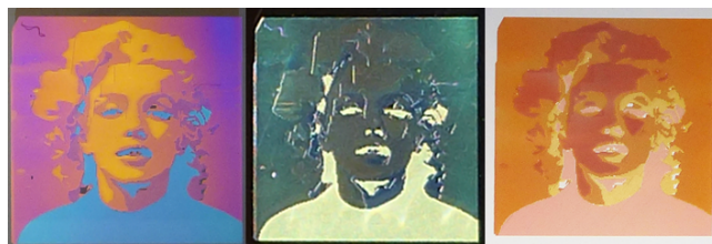
Figure 4. Color image printed with PICSLUP (1 x 1 cm), showing the dramatic color change depending on the illumination and measurement geometries. Left: Specular reflection mode ( 45^\circ:45^\circ geometry); center: Non-specular reflection mode ( 45^\circ:0^\circ geometry); right: Transmission mode ( 0^\circ:0^\circ geometry).
