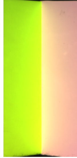
Figure 4. Observed color image of a fluorescent object (left) and a non-fluorescent object (right) under the artificial sunlight illumination. Interreflection effects appear in the region close to the intersection.
