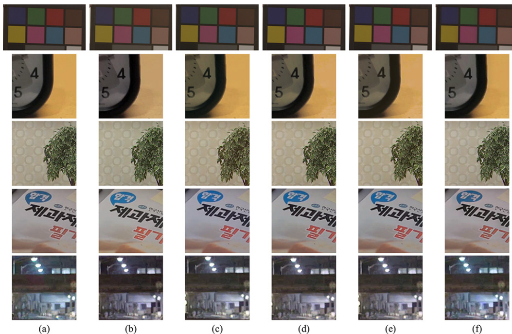
Figure 4. Enlargement of the images shown in Fig. 3: (a) left images (reference images), (b) right images, (c) color-matched right images by histogram matching with a weighted model, (d) color-matched right images by cumulative histogram matching, (e) color-matched right images by integrated color matching, and (f) color-matched right images by the proposed method.
