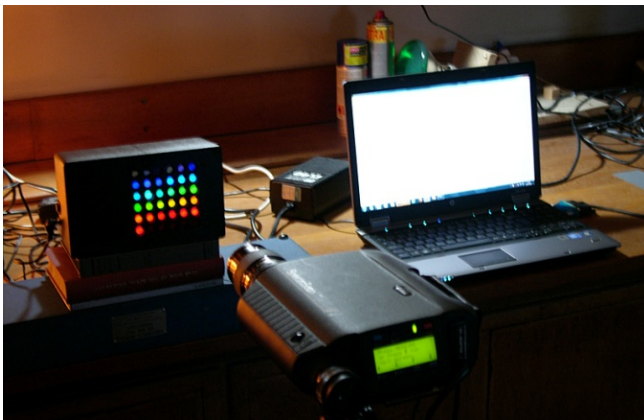
Figure 3. Laboratory setup for spectral measurement by PR-650 (foreground)
