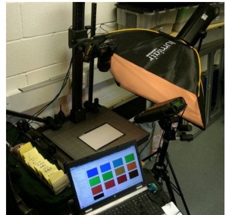
Figure 9. Camera with filter mounted on copystand with diffused flash lighting. Light reflected from white card was measured by PR-650 under PC control.
