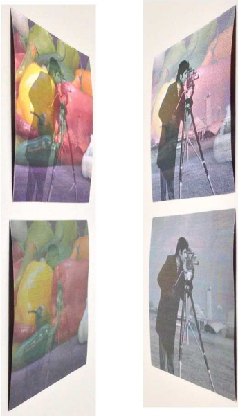
Figure 5. Comparing a printout as seen from the left (left images) and from the right (right images) side, with (bottom) and without (top) ghosting effects compensation [18].
