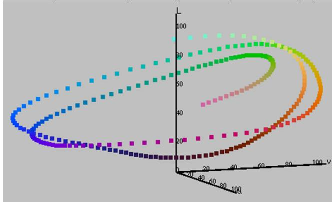
Figure 1. 256 primary colors produced by a CTRD (in CIELUV color space)
