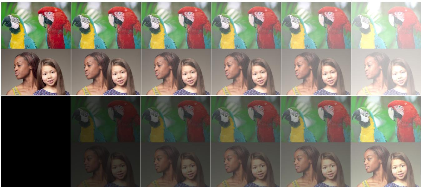
Figure 10. Simulation of sRGB images on an emissive display and a color tunable reflective display. Ambient light is zero on the left image and gradually increase to very bright on the right image.
