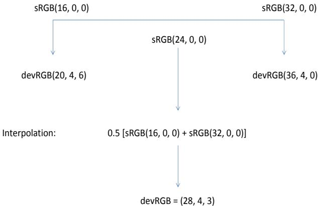
**Figure 2.** A 3-D interpolation example
