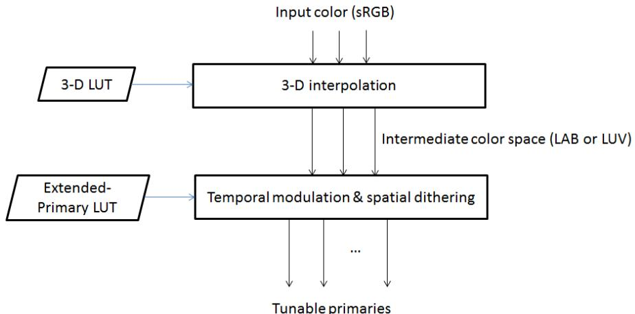
Figure 8. CTRD color rendering pipeline
