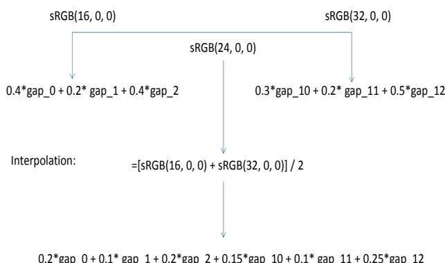
**Figure 3.** Transform an sRGB color to a multi-primary reflective display color using a 3-D interpolation method
