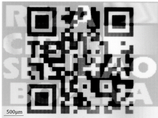
(a) Covert QR code recorded within the visible image on Nano-Media (Image is inverted)
