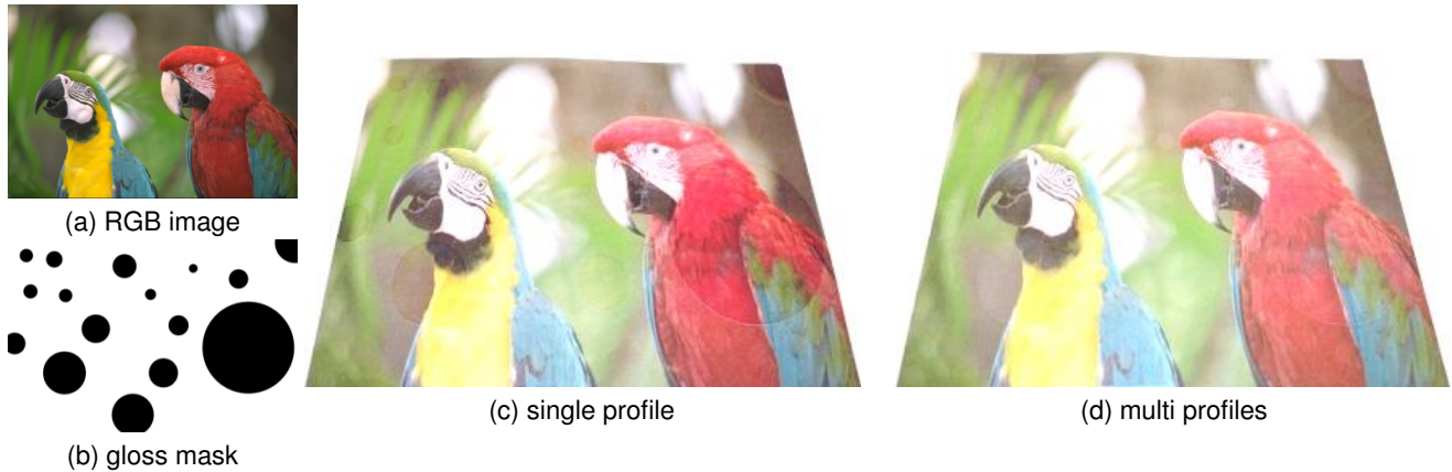
Figure 1. Image (a) is printed with two intended local gloss levels described by (b) where white corresponds to 'matte' and black to 'gloss'. In (c) the printout shows colour inconsistencies between varying gloss modes, while the printout in (d) shows colour consistent transitions, using our proposed multi profile workflow. For display purposes, the photographs of printouts (c) and (d) are rendered with exaggerated contrast.
