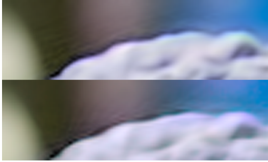
Figure 3. Comparison of a region between contourlets (top) and shearlets (bottom). The contourlet method has more prominent ringing artifacts compared to shearlets. The image has been enlarged to enhance the differences.
