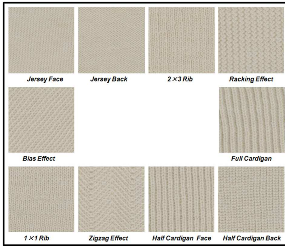
Figure 1. Scanned images of the woolen knitted samples representing various textures examined in this study
