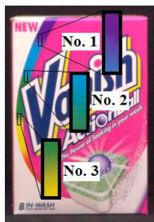
Figure 9: Spectral image with three extracted colour shadings. Each multispectral shading is numbered. Final multispectral shadings are the average of four columns.
