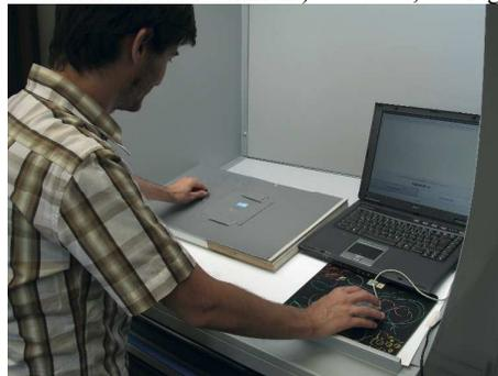
Figure 1. The sample colours are presented on a grey background. The computer on the right allowed for making the pair comparison judgments. The left hand rotates the turning wheel beneath the grey cardboard.
