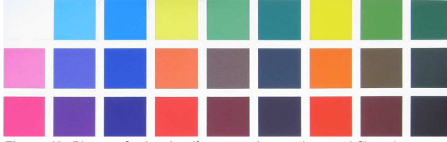
Figure 12. Picture of printed uniform samples on the metal film taken at an exposure of 1/250 s, with an aperture of F5.6.
