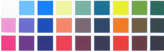
Figure 13. Picture of the corresponding printed uniform samples on paper taken at an exposure of 1/125 s, with an aperture of F5.6.
