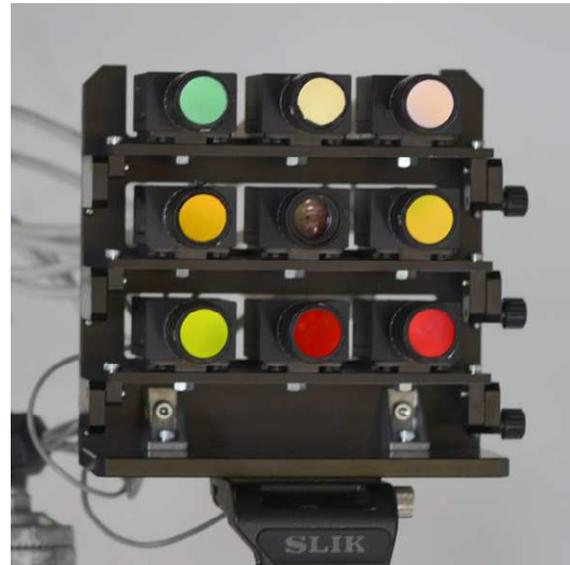
Figure 1. Eleven-band stereoscopic camera system.
