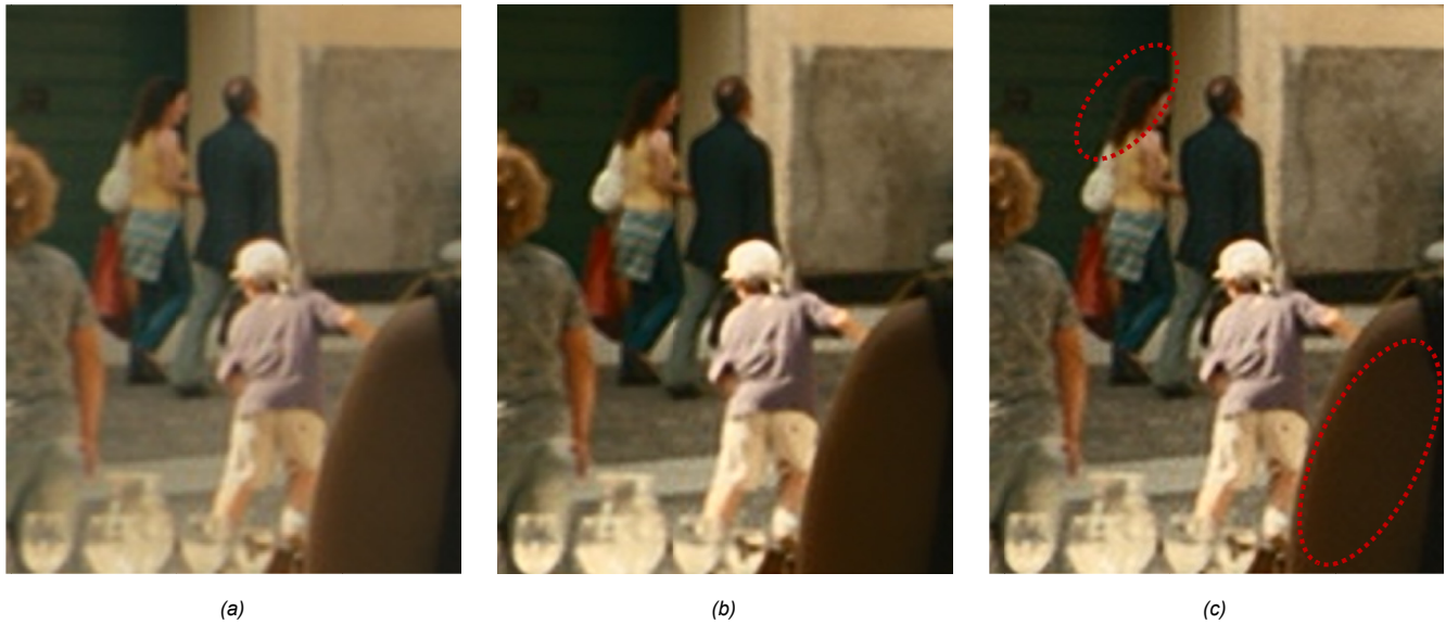
Figure 6. (a) Original, (b) results of the proposed method, and (c) results of a conventional method. The local contrast and clarity of object boundaries tend to increase while the other frequency components such as strong edges and flat regions are less affected. However, halo and random noise artifacts are resulted from the conventional method.
