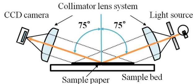
Figure 4. Apparatus diagram for measuring SR-PSF
