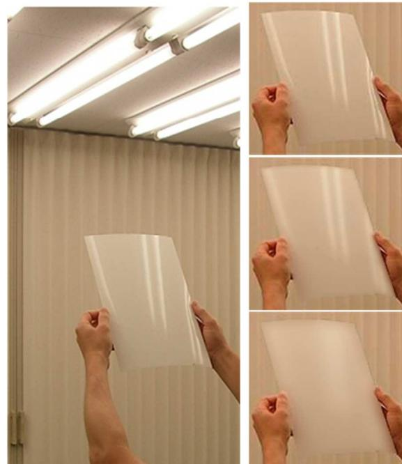
Figure 1. Scenes evaluating printing paper. The light sources are reflected on the curved paper. We can see different gloss levels from the images of the reflected light source. The upper right is a high glossy paper, the middle one is glossy and the bottom one is mat.
