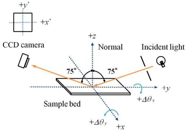
Figure 8. Coordinate system of measurement apparatus for SR-PSF.
