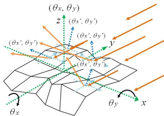
Figure 2. Schematic diagram showing macroscopic and microscopic facets on surface of flat paper.
