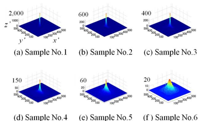
Figure 6. Measurement results of SR-PSFs. The maximum value of the  $z'$ -axis is 2000 in (a), 600 in (b), 400 in (c), 150 in (d), 60 in (e) and 20 in (f)
