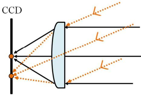
Figure 7. Schematic diagram of collimator lens system
