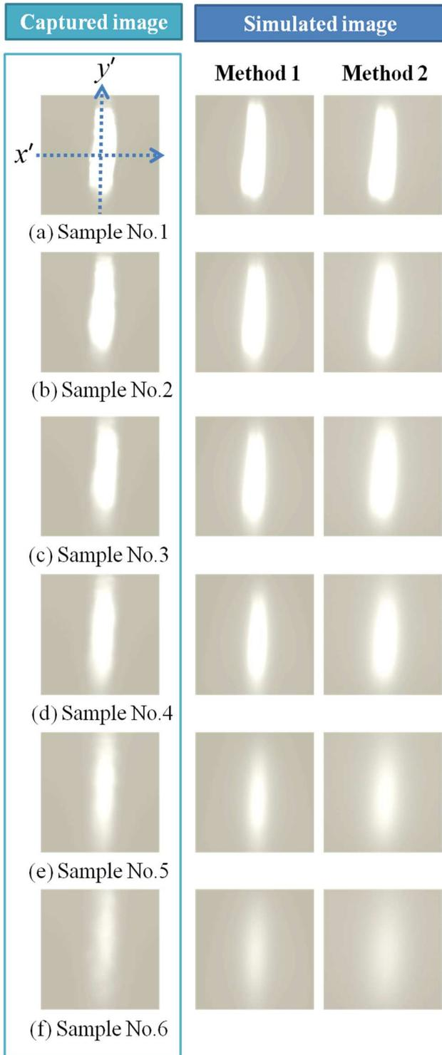
**Figure 12.** Simulated results of the paper gloss. From left to right, the figures show the captured images, the simulated images regarded macroscopic angle dependency as Method 1, and the simulated images regardless macroscopic angle dependency as Method 2.
