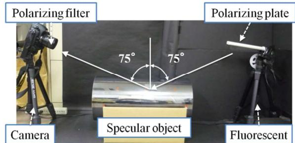
Figure 11. The photographing environment for the paper gloss simulation.
