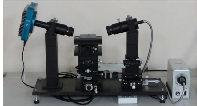
Figure 3. The measurement apparatus for SR-PSF
