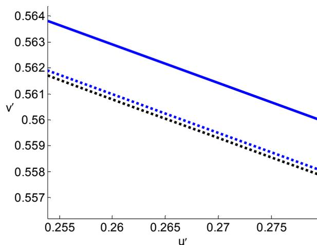
**Figure 7:** Detail of Figure 6 along the lower part of the  $B=0$  side of the CAT02 triangle. The solid blue line is part of the CAT02 triangle, the dotted blue line is part of the HPE triangle, and the dotted black curve is the CIE spectral locus.
