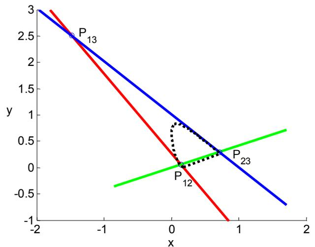
Figure 1: Response lines  $R=0$  (red),  $G=0$  (green) and  $B=0$  (blue), and red ( $P_{23}$ ), green ( $P_{13}$ ) and blue ( $P_{12}$ ) primaries in the  $x,y$  chromaticity diagram for the CAT02 matrix. The dotted curve is the CIE spectral locus and purple line.
