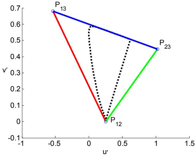
**Figure 4:** Response lines R=0 (red), G=0 (green) and B=0 (blue), and red (P<sub>23</sub>), green (P<sub>13</sub>) and blue (P<sub>12</sub>) primaries in the  $u',v'$  space for the HPE matrix. The dotted curve is the CIE spectral locus and purple line.
