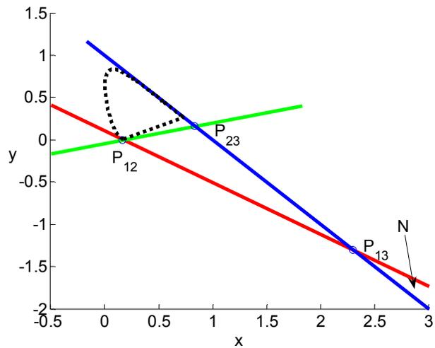
Figure 3: Response lines  $R=0$  (red),  $G=0$  (green) and  $B=0$  (blue), and red ( $P_{23}$ ), green ( $P_{13}$ ), and blue ( $P_{12}$ ) primaries in the  $x,y$  chromaticity diagram for the HPE matrix. The dotted curve is the CIE spectral locus and purple line. The letter  $N$  indicates the region where all the  $R$ ,  $G$ , and  $B$  responses are non-positive.
