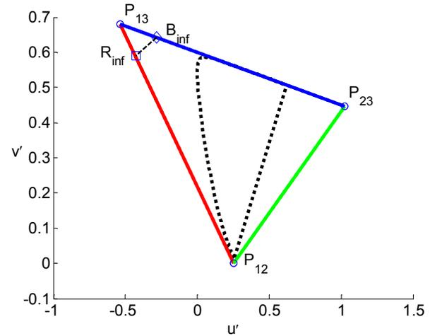
**Figure 5:** Response lines R=0 (red), G=0 (green) and B=0 (blue), and red (P<sub>23</sub>), green (P<sub>13</sub>) and blue (P<sub>12</sub>) primaries in  $u',v'$  space for the HPE matrix. The dotted curve is the CIE spectral locus and purple line. The points R<sub>inf</sub> and B<sub>inf</sub> are the limits in  $u',v'$  space when  $x,y$  values along the R=0 and B=0 lines, respectively, approach infinity in both directions.
