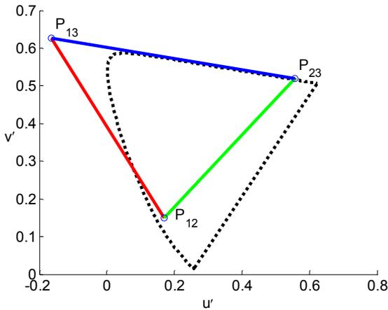
Figure 2: Response lines  $R=0$  (red),  $G=0$  (green) and  $B=0$  (blue), and red ( $P_{23}$ ), green ( $P_{13}$ ), and blue ( $P_{12}$ ) primaries in the  $u',v'$  space for the CAT02 matrix. The dotted curve is the CIE spectral locus and purple line.
