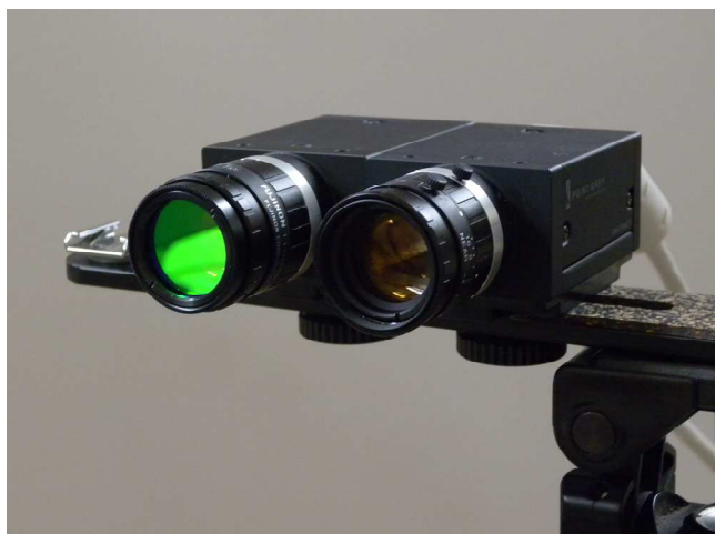
Figure 1. Six-band stereoscopic camera system. The interference filter is attached to the right camera.
