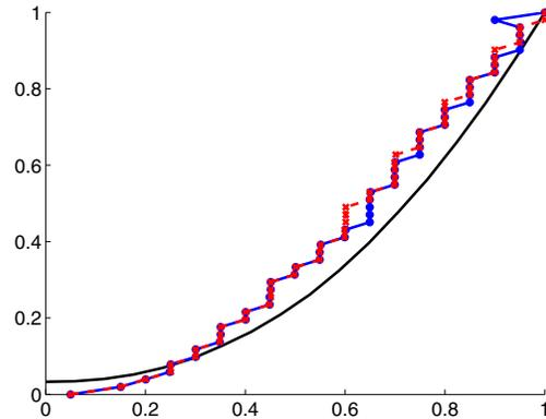
**Figure 8.** Two evaluations of the response curve of the 3-LCD projector with 50 luminance values and a discretization step of 0.05; the results are relatively consistent.
