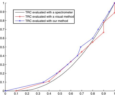
**Figure 6.** Tone response curve evaluation for the DLP projector by three different methods: Visual, webcam and spectrometer (the reference). We can see that our method is working pretty well with this set-up. The chosen discretization step was 0.1 for the evaluation of  $f$ . The results are similar to the observers.
