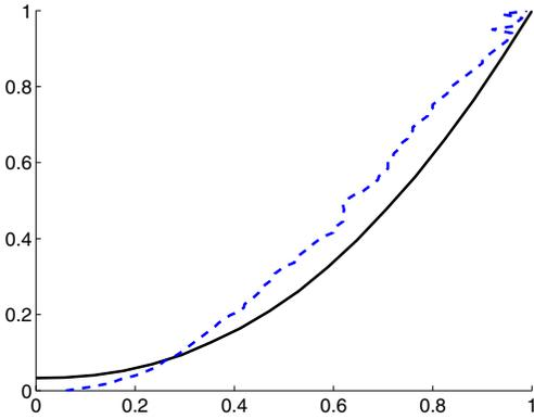
**Figure 9.** Evaluation of the response curve of the 3-LCD projector with 100 patches with a discretization step of 0.01. The method is relatively stable from values close to each other. We can notice some unconstancy on the high luminances.
