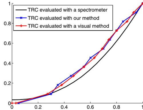
**Figure 7.** Tone response curve evaluation for the 3-LCD projector by three different methods: Visual, webcam and spectrometer (the reference). We can see that our method is working pretty well with this set-up. The chosen discretization step was 0.05 for the evaluation of  $f$ . The results are similar to the observers.
