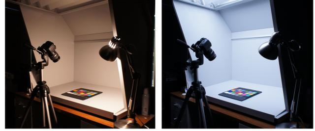
**Figure 5** Lighting and capturing setups using digital camera. Left: incandescent lighting geometry. Right: diffuse lighting geometry.
