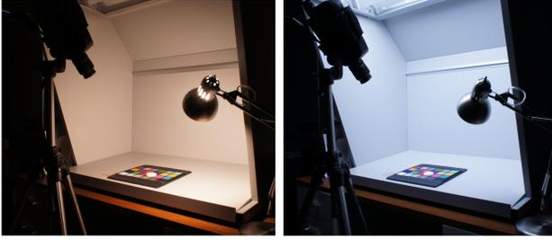
**Figure 3.** Lighting and capturing setups for measuring the spectral radiance by PR655. Left: incandescent lighting geometry. Right: diffuse lighting geometry.
