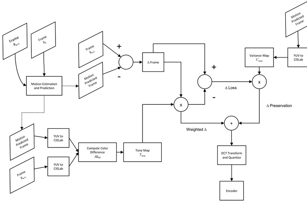
Figure 4. Modified video CODEC workflow for inter frame video coding with color difference compression
