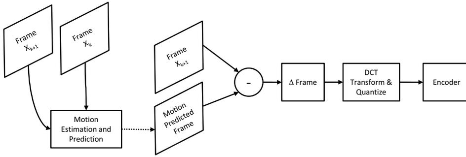
Figure 2. Baseline video CODEC workflow for interframe video coding
