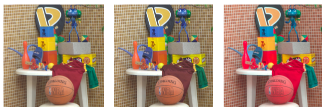
Figure 15. Hyperspectral image rendered for: (left) D65 illumination; (centre) optimum laser wavelengths; (right) Arius 3D colour laser scanner.
