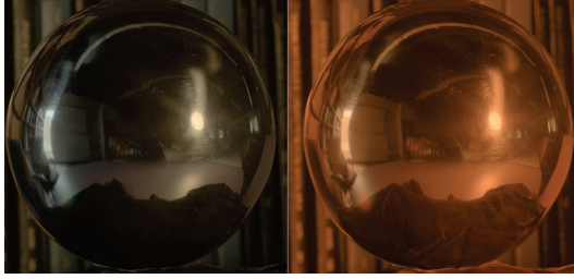
Figure 5. Images of the mirror sphere captured through the cyan (left) and yellow (right) filters of the multispectral camera system.
