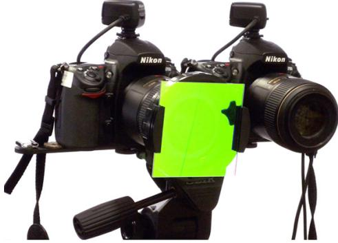
Fig.3: Stereo six-band camera system
