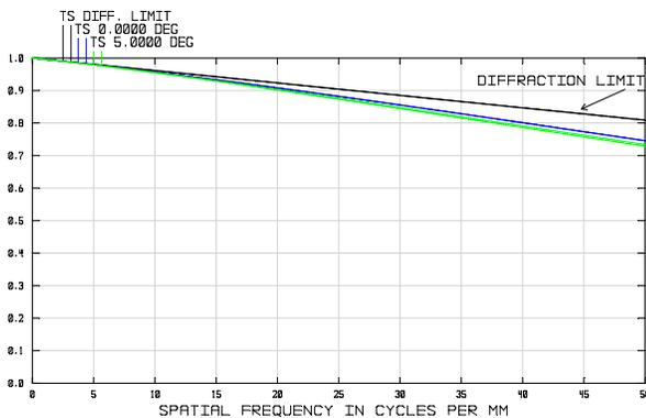
Figure 4. On-axis and 5° off-axis polychromatic MTF of the objective up to the Nyquist frequency
