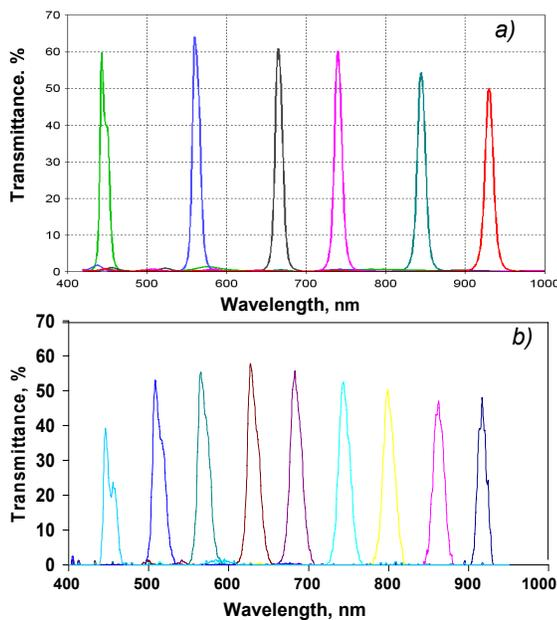
**Figure.7. a)** Calculated transmittance of a variable metal-dielectric filter with 21 layers. **b)** measured transmittance of a variable metal-dielectric filter with 21 layers.
