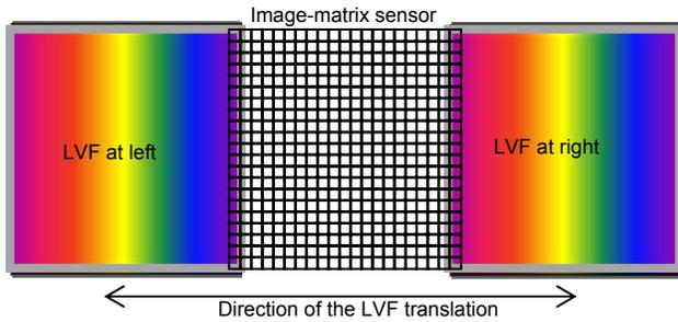
Figure 2. Image-matrix sensor and LVF edge positions. Each column of the image sensor colliding on a LVF strip is filtered at a selected wavelength depending on the filter position.
