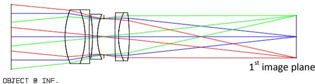
Figure 3. Layout of the objective with on-axis and extreme off-axis ray-tracing.
