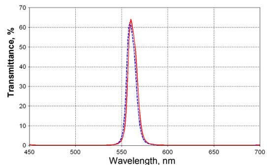
**Figure 8.** Calculated transmittance of a metal-dielectric filter centered at 560nm, illuminated at normal incidence (solid red curve) and with a convergent beam of semi-angle  $10^\circ$  (dashed blue curve).
