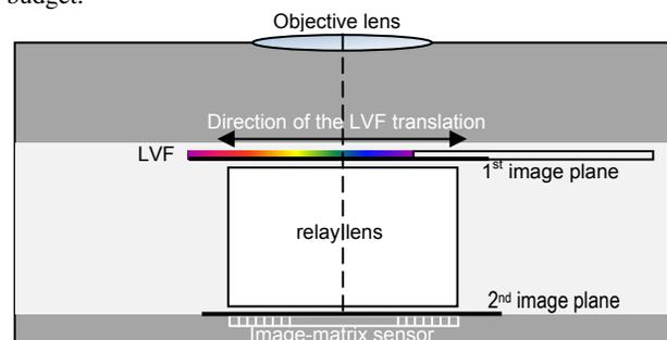
Figure 1. Cross sectional sketch of the spectro-photo/radio-metric camera. Each strip of the image on the 1<sup>st</sup> image plane is filtered by the LVF at a proper wavelength in order to return the spectral information. The filtered images are reproduced on the sensor by the relay lens. The whole spectrum is reconstructed strip by strip through LVF shifting.
