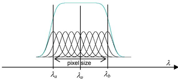
**Figure 9.** Spectral Transmittance of the LVF associated to a slit as large as a pixel.  $\lambda_p$  is the central wavelength of the band,  $\lambda_a$  and  $\lambda_b$  the boundary wavelengths. This bandpass does not consider the effect of the relay lens.
