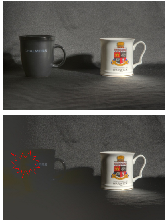
Figure 5: Tone mapped image of part of a scene after being captured with (top) 20 f-stops (bottom) 16 f-stops. Missing detail (and commercial opportunity) indicated in red.
