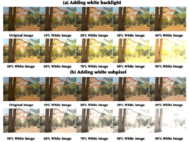
Figure 6. Comparison between the two simulations (The defined percent white here is from 0 to 90% with an interval of 10%; the test image is Cemetery Tree.)
