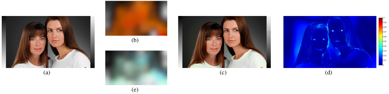
Figure 4. The input image (a) is described using the concept of optimal primaries and (9 \times 16) segments, shown in (c). In (b) and (e) the backlight of field 1 and field 2 is shown. The resulting colour error map in \Delta u'v' is shown in (d).
