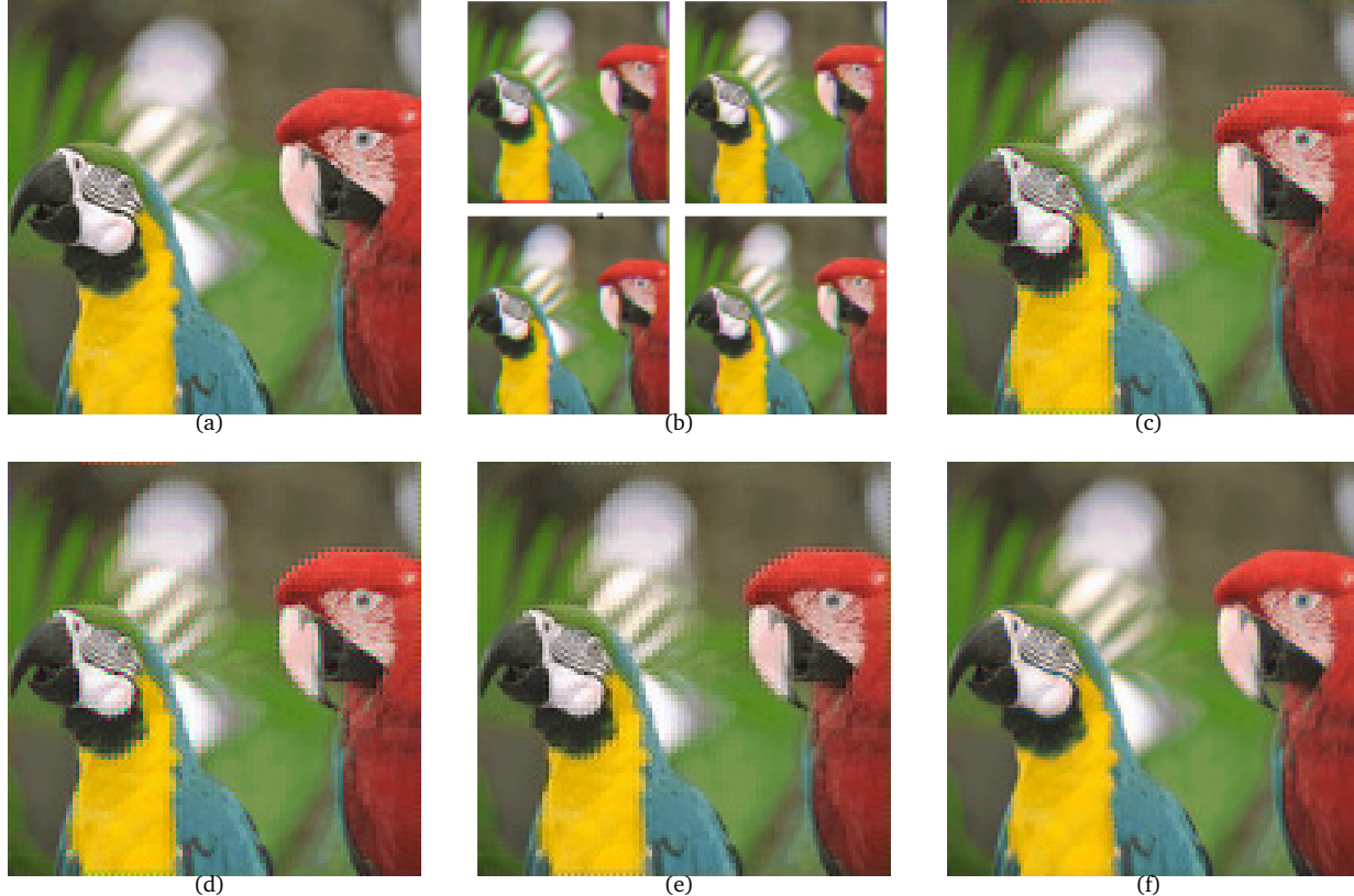
Figure 2. Illustration of significance of chrominance geometry. (a) Original hi-res image (128×128). (b) Four sample lo-res images generated synthetically (64×64). (c) SR performed on RGB channels independently. (d) SR performed on luminance channel only (chrominance channels interpolated in a simple manner). (e) SR performed independently on luminance and chrominance channels. (f) SR performed with chrominance geometry-sensitive regularizer - proposed method.
