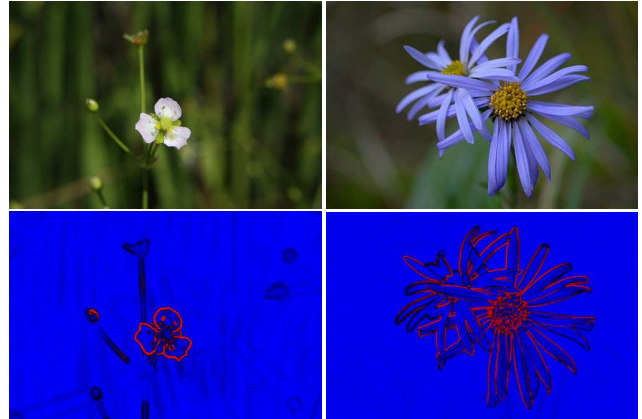
Figure 3. Some natural images and magnitude of the Di Zenzo gradient (in blue are values near 0 and in red the high values)
