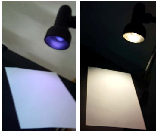
Figure 2. Simulated CAT effect. Un-adapted on the left, adapted on the right.
