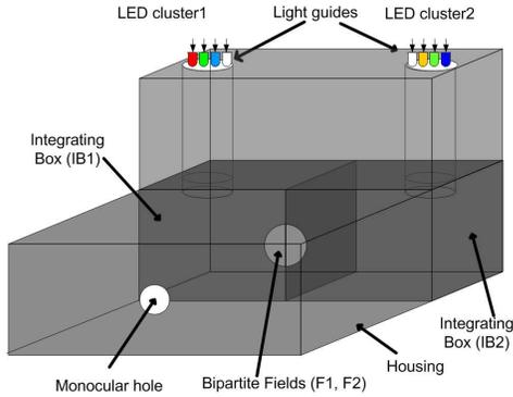
**Figure 5.** Configuration of the Observer Calibrator Prototype
