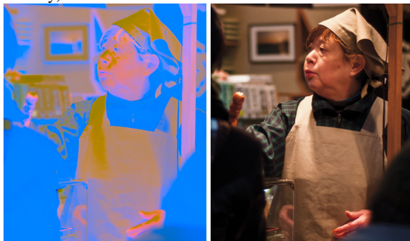
Figure 5. A scrambled image (sRGB preview) and the re-constructed image in the target device's RGB space (sRGB preview) with a simple scrambling over a CLUT of size 33^3 .
