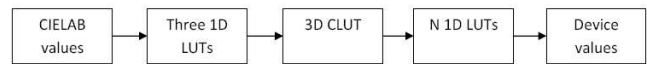
Figure 2. Order of transforms in an inverse tag of a typical ICC profile
