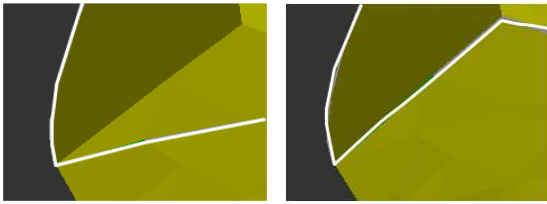
Figure 4. Estimated cusp (white line) without (left) and with (right) surface curvature criterion for an EBU display
